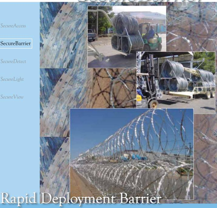
The system is designed to provide rapid deployment – 75 meters (246 ft.) to 300 meters (984 ft.) of barbed tape/razor wire coils which can be deployed in seconds. Depending on
